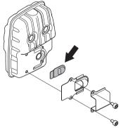
If the mesh is frequently blocked, this can be a sign that the performance of the catalytic converter is impaired. Contact your dealer to inspect the muffler. A blocked mesh will cause the machine to overheat and result in damage to the cylinder and piston.
