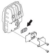
If the muffler on your machine is fitted with a spark arrestor mesh this must be cleaned regularly. A blocked mesh will cause the engine to overheat and may lead to serious damage.
