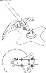
Check that the guard is undamaged and not cracked. Replace the guard if it has been exposed to impact or is cracked.
