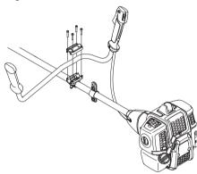
Fit the protective sleeve as shown in the diagram.
